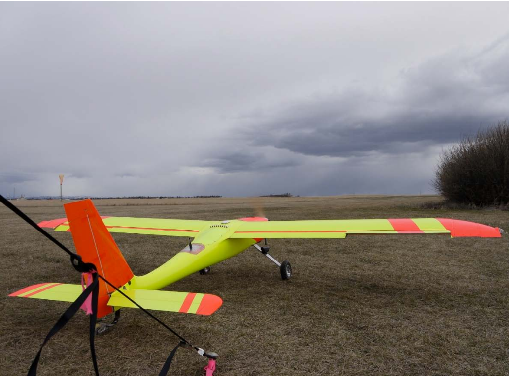
Canada's Stratus Aeronautics has built its own drone that can fly magnetic surveys to search for mineral deposits. Right now, most surveys are done using conventional aircraft.
